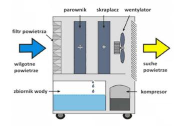
This dehumidifier controls humidity by forcing excess moisture to condense from the air into the unit as it passes over the cooling elements. Contact with this cold surface causes the moisture in the air to condense. This condensed water the drains safely into the water tank. The dried air then passes through a warmed coil where it is slightly warmed and reenters the room at a slightly elevated temperature.
